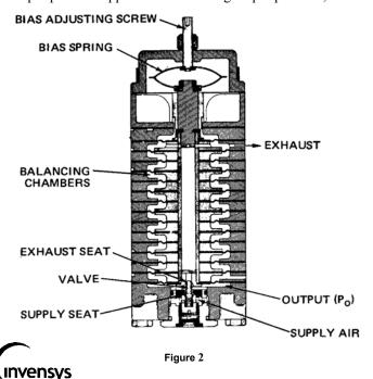
center assembly will be returned to the balanced position, permitting the supply seat of the valve to close, throttling the flow of supply air.
