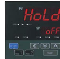
► To hold currently running program: "Hold=On"
