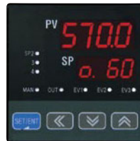
► Display of Control Output status (%FS of output)
