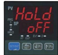
► To hold currently running program: "Hold=On"
