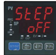
► To jump to next program segment immediately: "Step=On"
