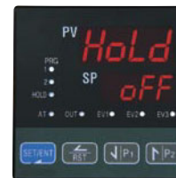
► To hold currently running program: "Hold=On"
