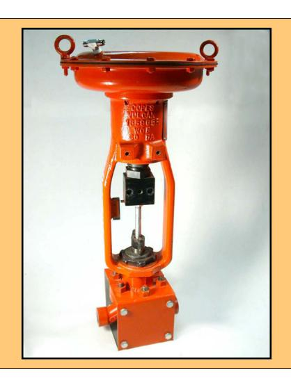
A Copes-Vulcan Type 700 Actuator with stem block coupling is shown in the photo on the left. These instructions will provide the information necessary to mount the ABB type TZID-C or TZID-C200 Positioner on this Actuator as well as Fisher 657/667 type Actuators.
