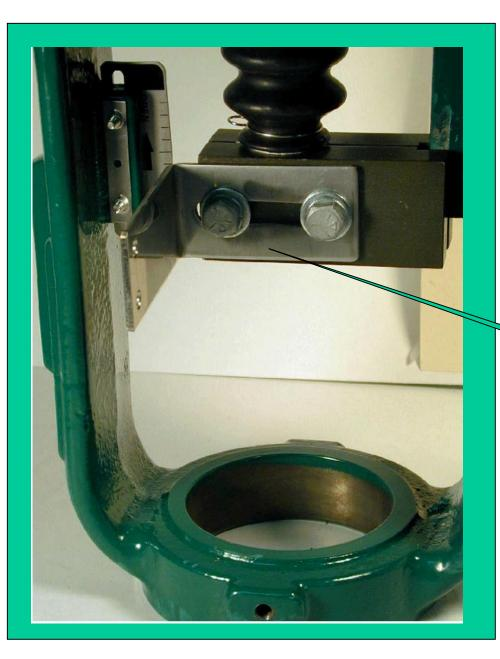
1. With the actuator mounted on the valve and the valve stem threaded into the split block coupling to the appropriate depth, install bracket, Item 1, onto the stem coupling block as shown using the bolts supplied with the coupling block. Torque the stem coupling bolts to the value specified by Fisher.
