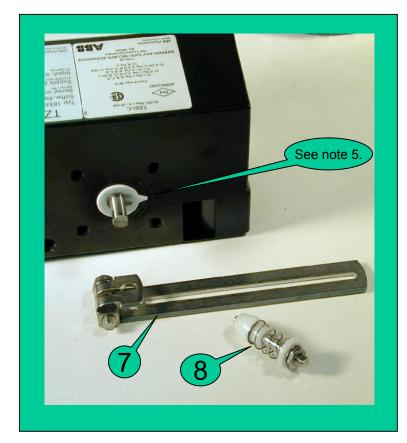
5. Mount the spring loaded slider assembly onto the positioner drive lever at a radius marking equal to or a little less than the valve stroke. The markings on the drive lever are in mm.
