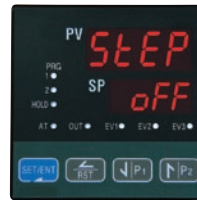
► To jump to next program segment: Step = On
