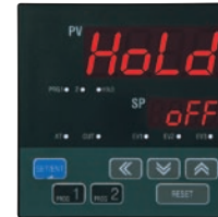
► To hold currently running program: "Hold=On"
