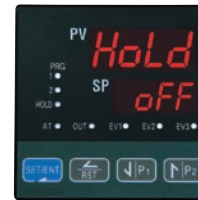
► To hold currently running program: "Hold=On"
