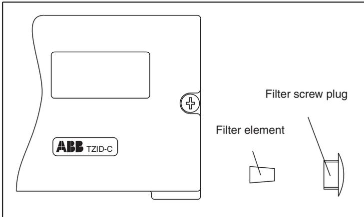
**Fig. 37 Filter screw plug (right side of case)**
