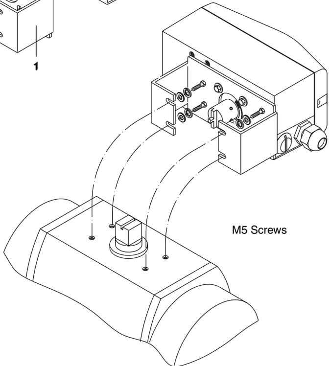
**Fig. 18 Attach TZID-C to actuator**
