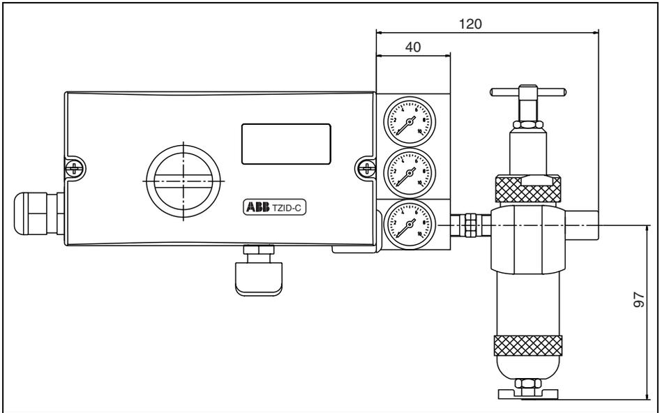
**Pressure gauge block with filter regulator**
