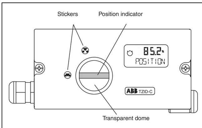
**Fig. 26 TZID-C with mechanical position indicator**
