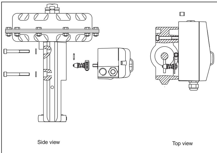
**Fig. 19 Integral mounting to valve 23/24, 23/25**
