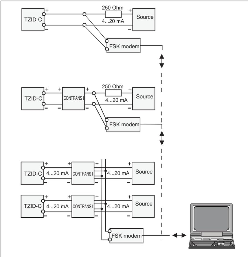
**Fig. 5 Communication via FSK Modem**
