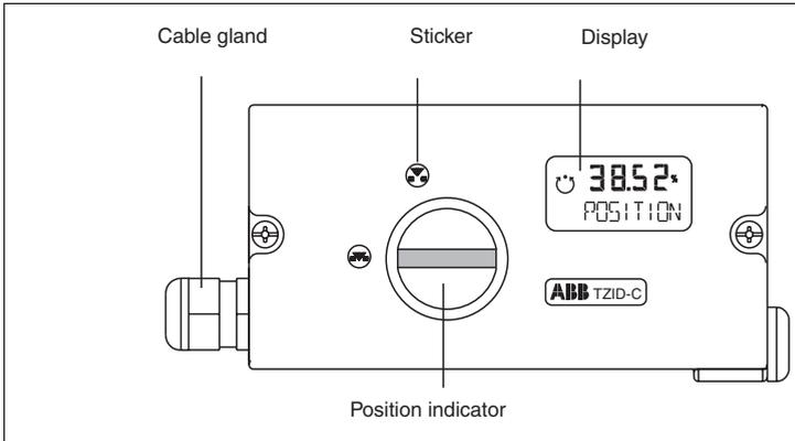
**Fig. 1 TZID-C positioner, closed**
