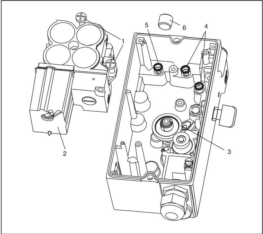
**Fig. 34 Replacing the I/P module**
