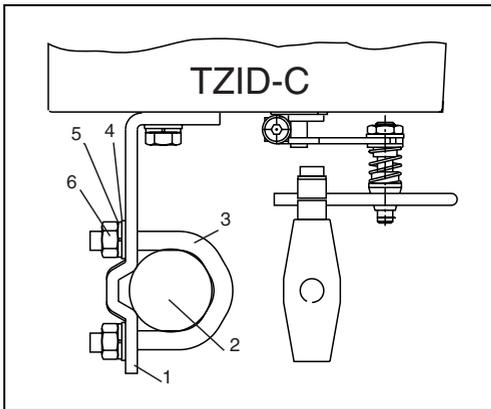
**Fig. 13 Mounting to columnar yoke**
