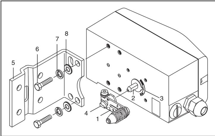
**Fig. 11 Mounting lever and angle bracket to TZID-C**
