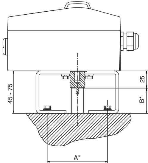
\*) Dimensions A and B depend on rotary actuator size
