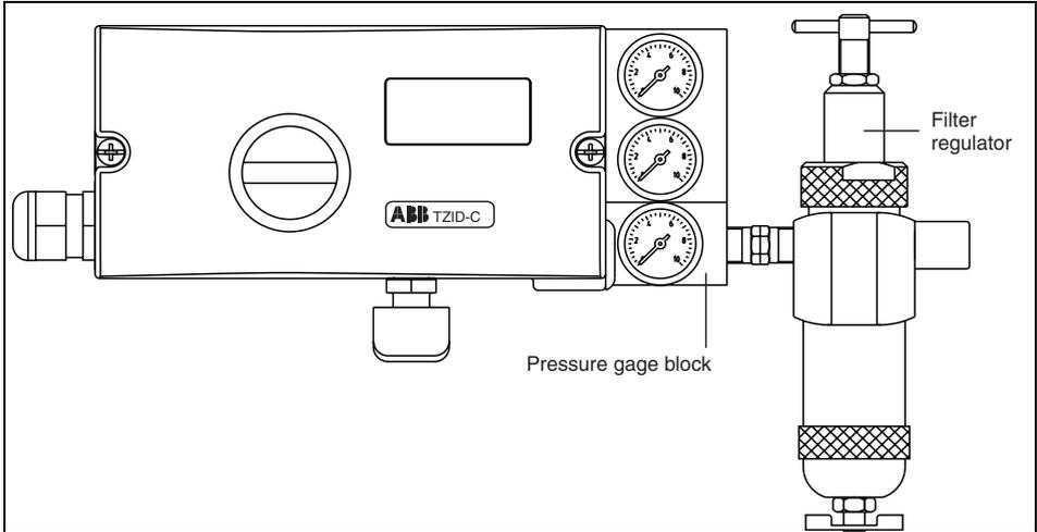
**Fig. 32 Pressure gage block with filter regulator**
