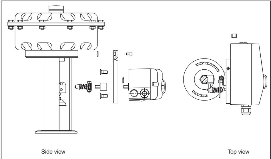
**Fig. 20** Integral mounting to valve 23/26
