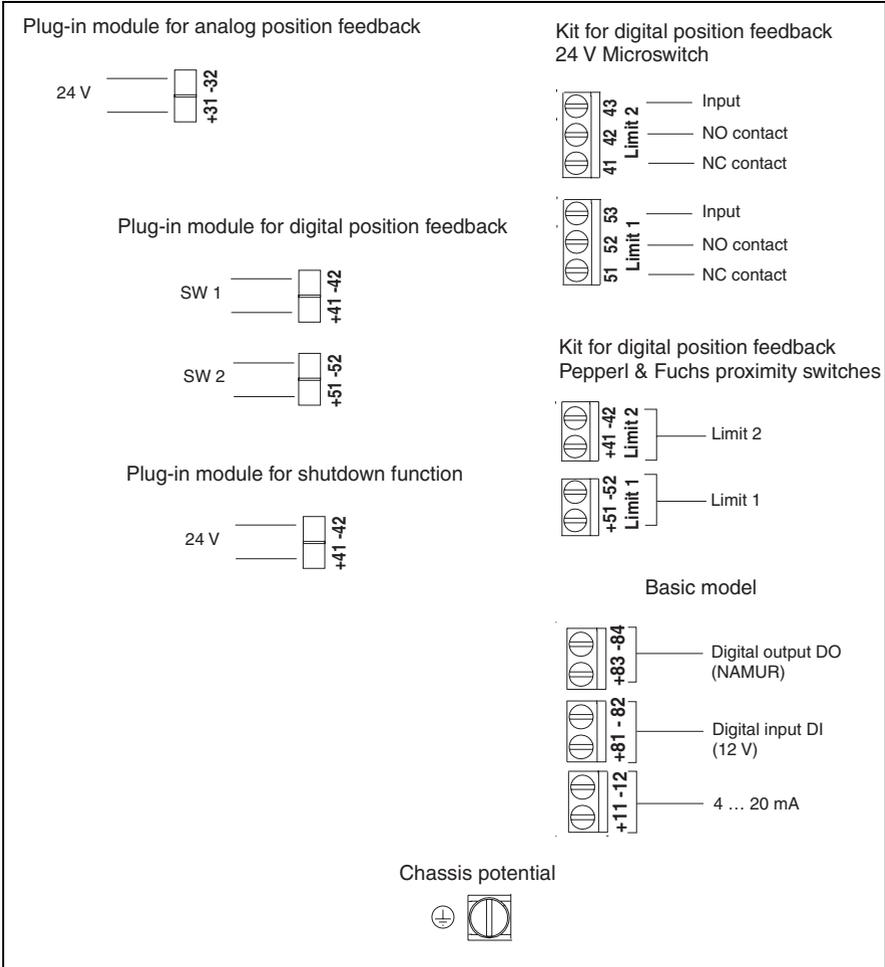
**Fig. 24 Terminal assignment**
