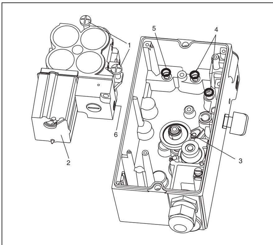
**Fig. 39 Filter element in I/P module**
