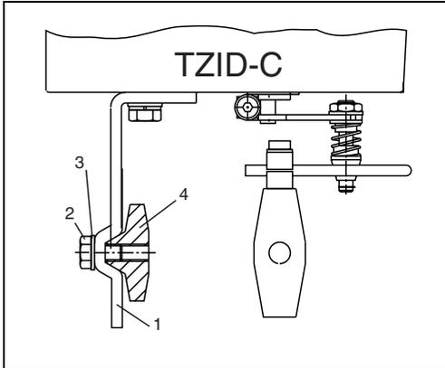
**Fig. 12 Mounting to cast iron yoke**
