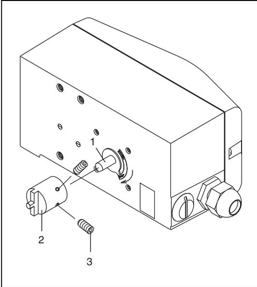
**Fig. 16** Mounting adapter to positioner
