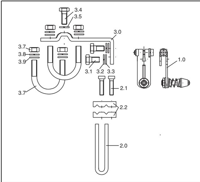
**Fig. 8** Mounting kit for linear actuators
