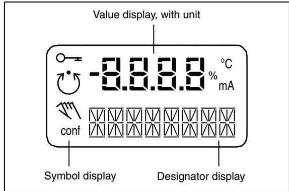
**Fig. 35** Liquid crystal display
