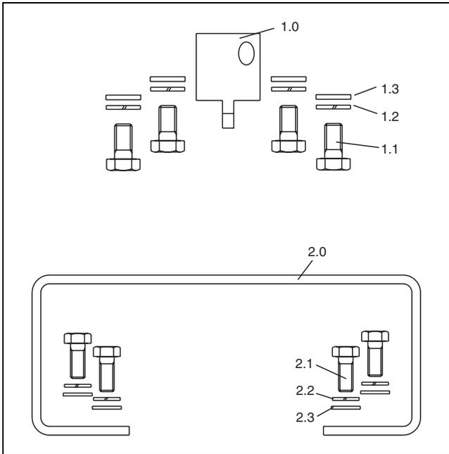
**Fig. 15 Mounting kit for rotary actuators**
