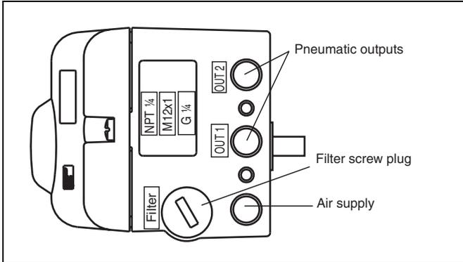
**Fig. 21 Pneumatic connections**
