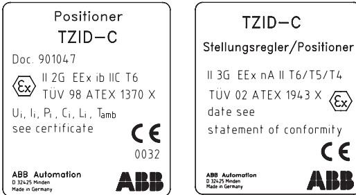
Fig. 1 Type plate indicating the degree of explosion protection
