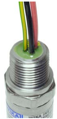
1/2" male conduit with 6 foot flying leads and factory epoxy seal
