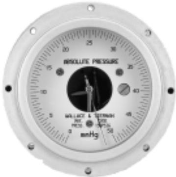
For routine test, laboratory, and production uses, this gauge gives accuracy and compact size. Its mechanism is sensitive yet rugged. And it offers high accuracy at low cost. Available in ten standard ranges, the Series 300 is convenient to use. Absolute pressure is applied to the case and readout is direct, without barometric or temperature corrections. Readings are referred to zero absolute.
